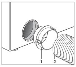
Install the connector, 1, with the exhaust hose or pipe, 2, to the dryer.
